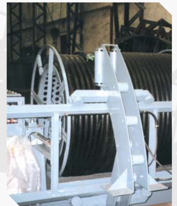
Wide cable reel with drive cable device.
